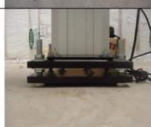
**Example** PT3 fastened to anchor plate.
